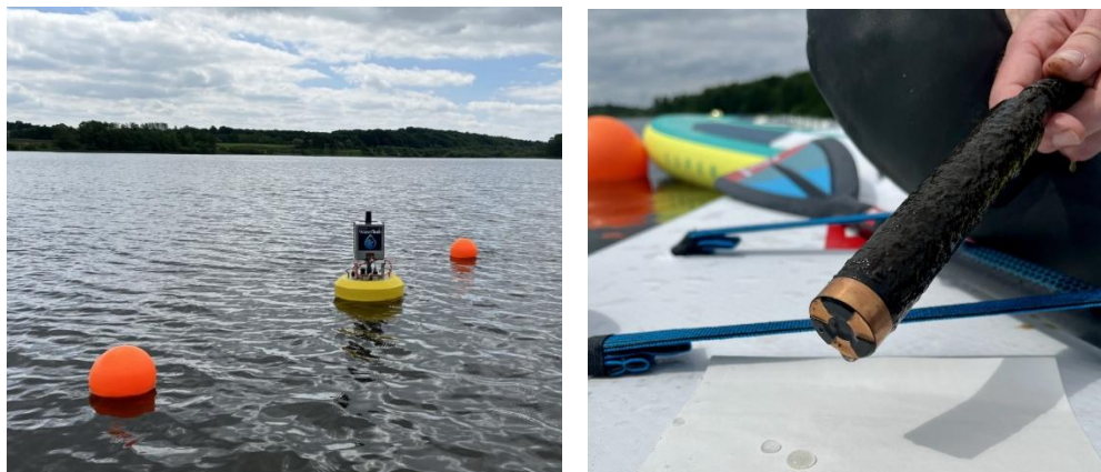
Fig. 1. Example of a data buoy (left) produced by WateriTech. Here, several OPTOD optical oxygen and temperature sensors (right) are placed at fixed depths, where the number of sensors and their placement is adapted to the individual system.
